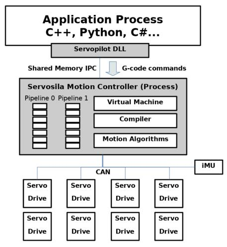
Internally, *Motion Controller* process has a *Pipeline 0* and a *Pipeline 1* for receiving G-code commands from an *Application Process*. The pipelines are cyclic buffers of a fixed size. There are two pipelines so that two independent streams of G-code commands could be executed in parallel if needed. When submitting a new G-code command, an *Application Process* may choose to append the command to one pipeline or the other, or to replace commands in a pipeline with a new set of commands.
