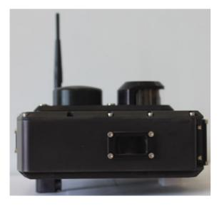
Since the robotic heads combine a high-performance computer and a set of sensors in the same package, the amount of cabling is significantly reduced, installation simplified and maintenance streamlined. The robotic heads can be also taken off the robots and used as desktop testbed computers by developers of onboard software; an HDMI monitor port and a keyboard port are provided to simplify desktop-style use.
