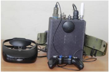
A portable operator control unit, or OCU, complements Servosila Robotic Heads with a remote control functionality. The unit is a passively cooled computer with a radio modem and a battery included into a water-tight enclosure.
