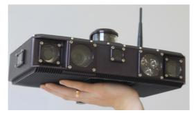
The robotic heads are highly integrated, sensor rich, passively cooled, watertight yet powerful computers designed to serve as centralized control nodes of mobile robots. The robotic heads feature an internal DC-to-DC power regulator that enables them to draw power from onboard batteries or power generators.
