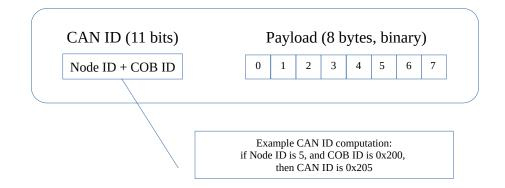
All types of messages consist of just two components, a **CAN ID** and a binary **Payload**.
