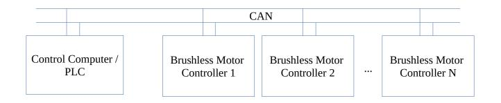
Up to 126 Servosila brushless motor controllers can be connected to the same CAN bus instance if a control computer/PLC has a hardware CANbus interface. Linux SocketCAN API can be used to develop software that sends commands to Servosila controllers or receives telemetry back from the controllers.
