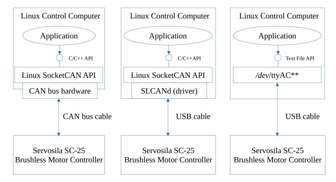
Linux SocketCAN API can be used to develop software that sends commands to SERVOSILA controllers or receives telemetry back from the controllers.
