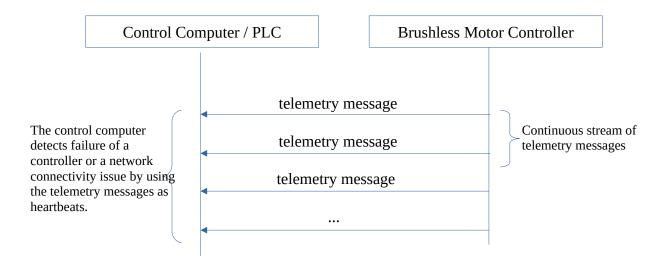
Servosila SC25 Brushless Motor Controllers continuously (periodically) send telemetry messages<sup>3</sup> back to a parent control system. The interval between telemetry messages is configured via the "Servoscope" software tool. The telemetry messages are sent asynchronously, and are not synchronized to commands or requests coming from a control computer.
