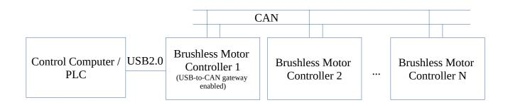
In this network architecture, it is allowed to connect third-party CAN devices to the network of brushless motor controllers. In such a case, the control computer communicates to the third-party devices via the USB-to-CAN gateway function in the same way as it communicates to the brushless motor controllers themselves.
