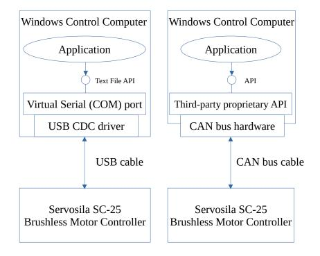
As Windows 10/8/7 systems do not have such a unified CANbus API, the ways for a control system's software running on Windows to interact with Servosila brushless motor controllers include:
