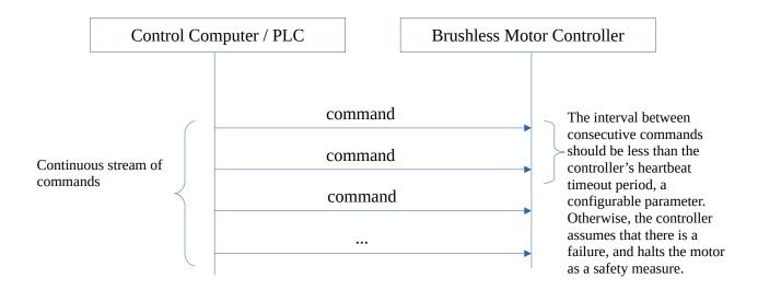
The control computer is expected to *continuously* send commands<sup>2</sup> to each of the Servosila SC25 Brushless Motor Controllers on the network. If such a continuous stream of commands suddenly stops coming to a motor controller, the controller assumes that there is a network fault or a failure in the parent control system. In such a case, the controller stops its motor as a safety measure, and might enable a brake function depending on configuration settings.
