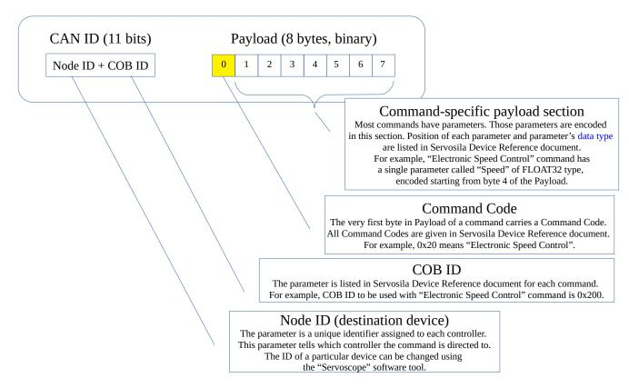
See sample C++ projects slcan-esc-command and canbus-esc-command for details on how to encode and send out a command to a Servosila SC-25 Brushless Motor Controller.
