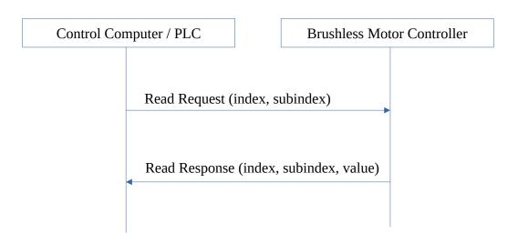
To identify a parameter of interest, the control computer uses an [Index:Sub-Index] pair of numbers. A list of all parameters, their indices, sub-indices and data types is given in a Servosila Device Reference document.
