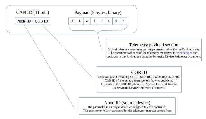
See sample C++ projects slcan-telemetry and canbus-telemetry for an example of how to receive and decode a telemetry message coming from a Servosila SC-25 Brushless Motor Controllers.
