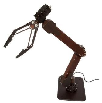
Servosila Robotic Arms are attachable payload modules for mobile service robots or other robotic platforms. The robotic arms are typically mounted on a chassis or a torso of a mobile robot and powered by an on-board power supply system of the host robotic platform.
