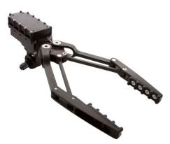
Servosila Robotic Arms are equipped with either a rotating or a non-rotating gripper optimized for grabbing objects from the ground or from various heights. Opening doors by rotating the door handles is a key design use case.
