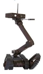
An unregulated DC power supply is all that is required to power a Servosila Robotic Arm on board of a mobile robot. Since most mobile service robots are powered either by a battery or by a power generator (including hybridelectric), the available on-board electric power might be scarce or unstable. Servosila Robotic Arms have special provisions that enable them to operate under such challenging conditions.
