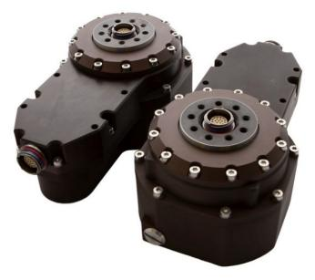
The main components of any Servosila Robotic Arm are servo drives that actuate each degree of freedom of the arm. Designs of the servo drives are based on a harmonic drive technology and a field-oriented BLDC motor control principle.
