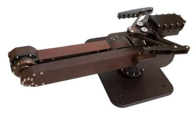
When not in an active use, Servosila Robotic Arms can be folded into a very compact form that doesn't occupy much space on the top of a robotic chassis or on the side of a torso. This feature protects the robotic arm of a mobile robot in case of an unexpected collision with an obstacle or whenever a rough terrain is encountered by the mobile robotic platform. The compact folded form also comes handy during transportation.
